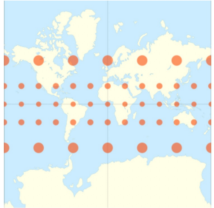
The Mercator projection with Tissot's indicatrix of deformation.
